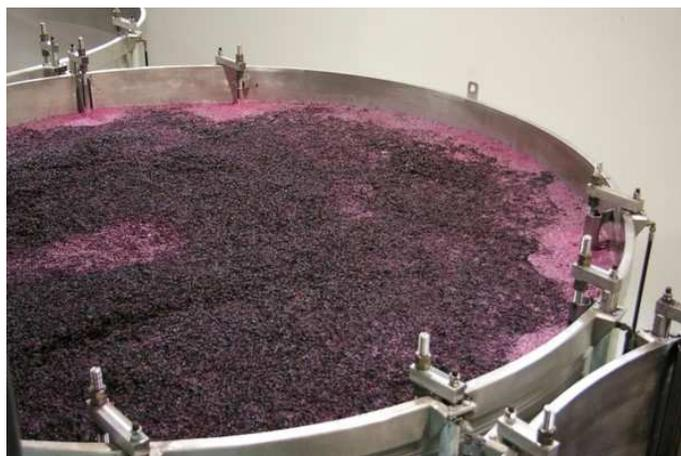
2200+ Bottles of Wine Enter Fermentation. CO<sub>2</sub> bubbles will take the skins to the top forming a cap. Greater contact between the skins and the must needs to be enhanced.
