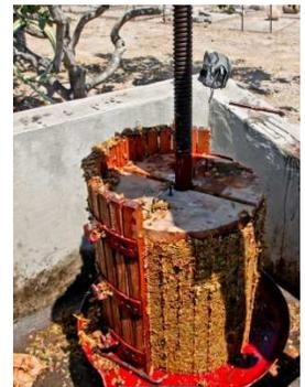
Simple press. Pressure is applied from the top and juice escapes through the spaces between the wood slats. What remains in the press is called pomace.
